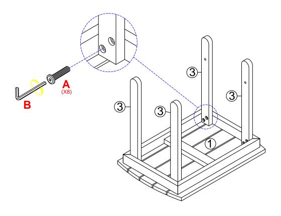
STEP 2: Attach 3 onto 2 using the bolts (A), tighten it up by using an allen key (B)
